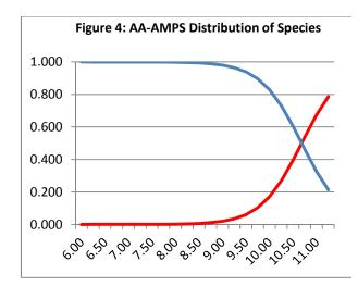
pH has a similar impact on polymer dosages for scale inhibition. The first time the author encountered the need to correct the dosages and models for speciation was in the development of a model for calcium phosphate scale inhibition by AA-AMPS (copolymer of acrylic acid and 2-acrylanmido-2-methylpropanesulfonic acid).
